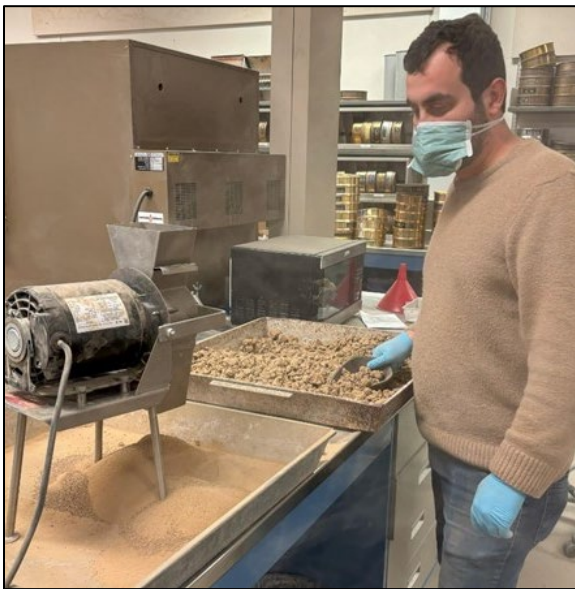
Figure 3.17 Grinding of clay soil lumps.
