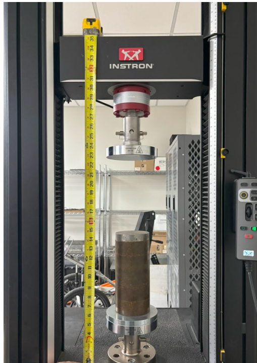
Figure 3.8 Instron testing device for UCS Testing
