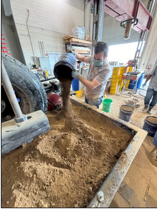
Figure 3.19 Placement of clay soil in steel box Figure 3.20 Compacted clay soil layer.
